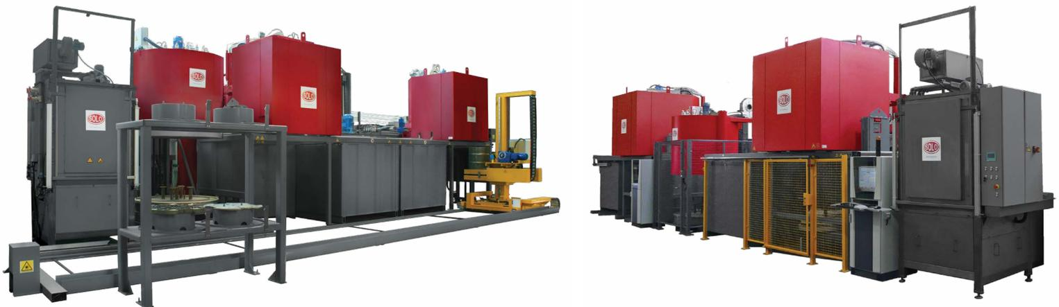
**Fully automatic SOLO® Profitherm furnaces lines, 1050°C**
